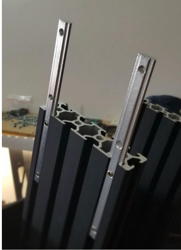
Linear 3030 connectors installed in the extension profiles.
