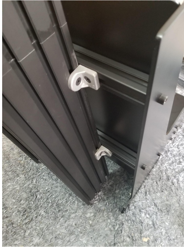
L-bracket connection at the lower rear seat structure.
