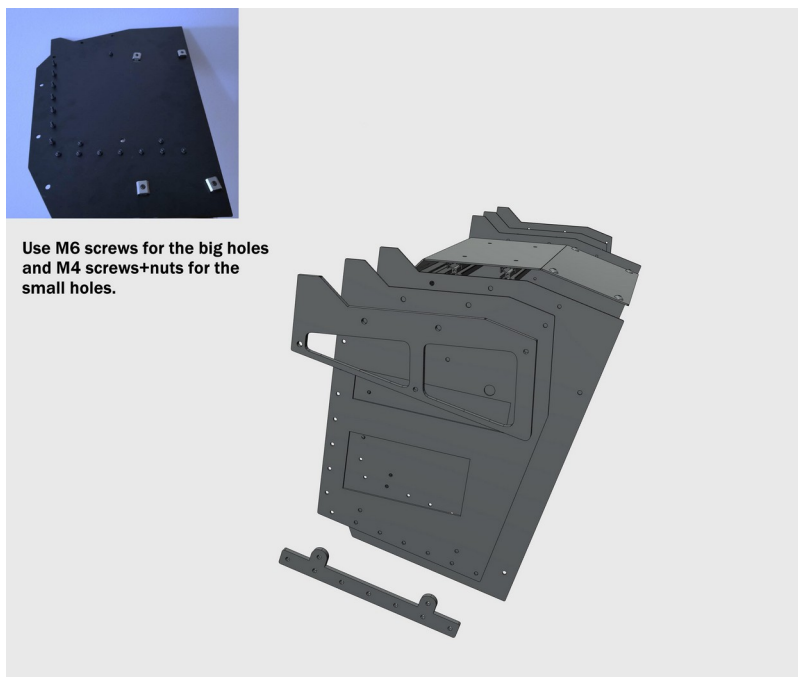
Rear panel and profile connection detail.
