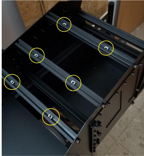
Required profile and fastener positions inside the parachute-box assembly.
