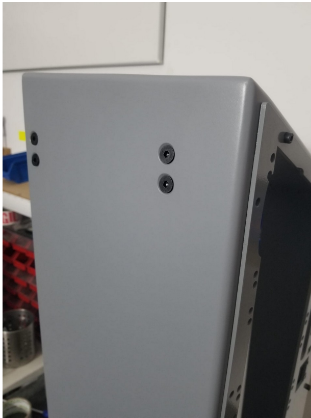
Flat-head screw installed through the console side panel.
