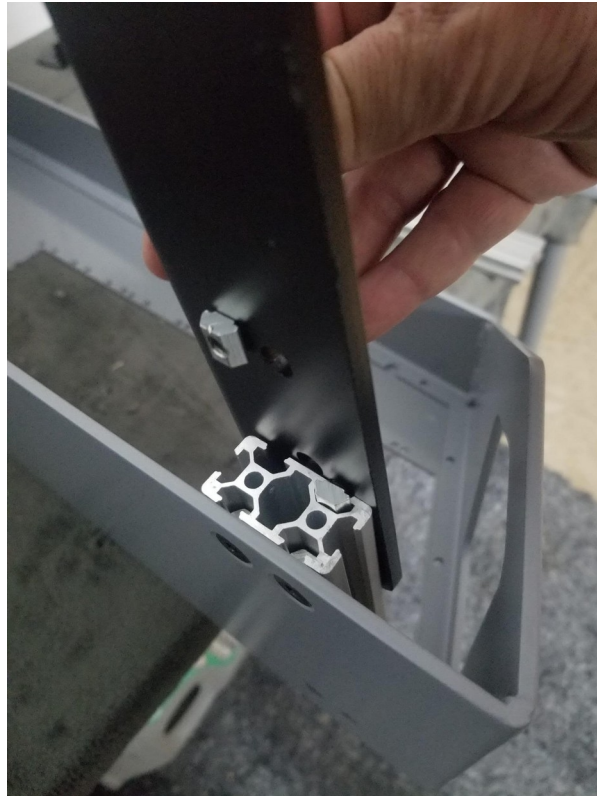
Bracket sliding into the 2040 profile groove.
