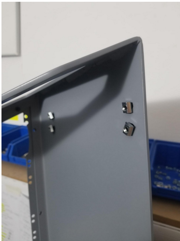
T-nut started on the rear side of the panel fastener.
