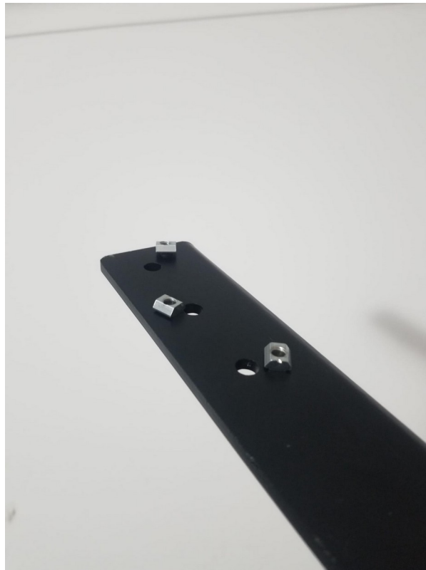
T-nuts started on the bracket screws.
