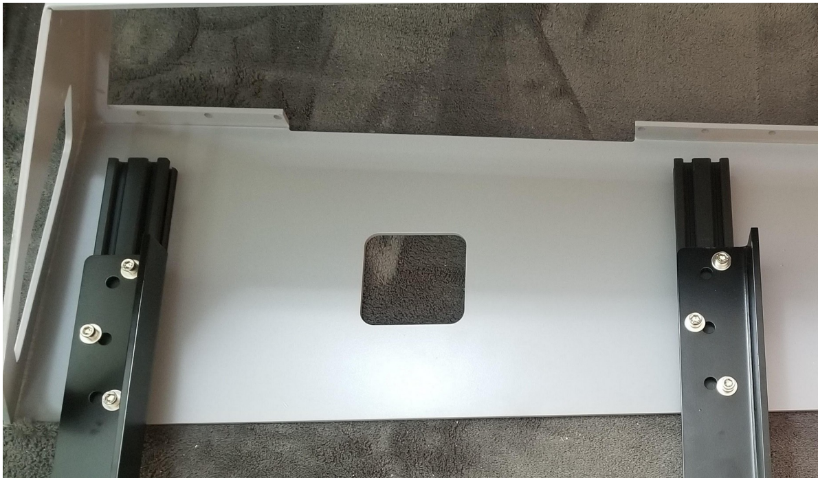
Three brackets positioned on the console profiles.
