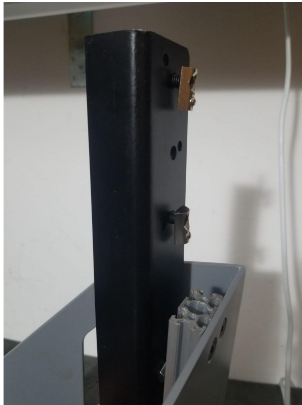
Console attached to the chassis through the three adjustable brackets.
