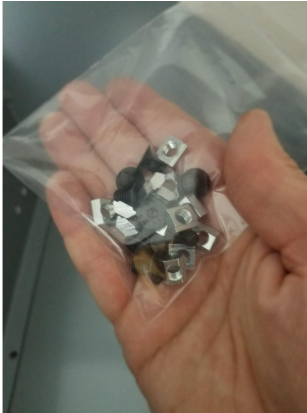
M6 T-nuts and flat-head screws used at the side panel.
