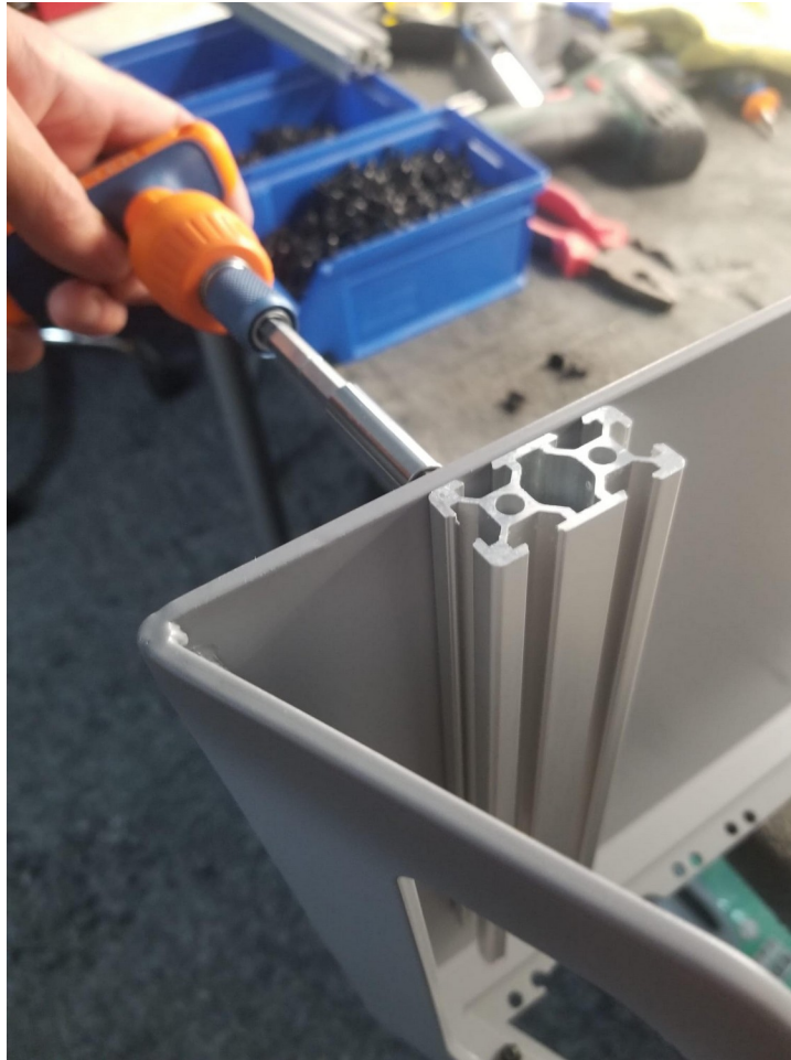
Profile groove entering the preloaded panel T-nuts.
